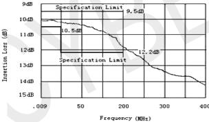
Fig.1 Typical Insertion Loss VS Frequency
