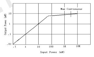
Fig.2 Typical Limiting Characteristics
