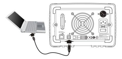
After successful connection, turn on the instrument and a "Found New Hardware Wizard" dialog box appears. Please follow the instructions to install the "USB Test and Measurement Device (Agilent)" on the PC. See the figure below.
