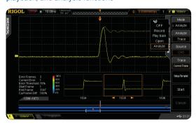
Serial bus trigger and decoding functions (supporting RS232/UART, I2C, SPI and CAN)
